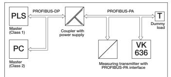
Fig. 2. Communication by PROFIBUS-PA interface.
